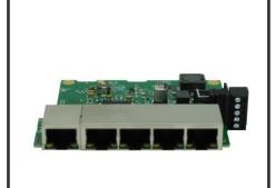
Embedded format, takes up minimal space, with mounting holes connected to Functional Earth
