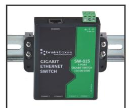
Integral wall mount option can be used with MK-048 clips to allow DIN rail mounting
