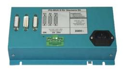
The **PG-Port Multiplexer** permits simultaneous, parallel connection of two devices to the programming interface of a SIMATIC S5. You can connect programming devices, text displays, operating units and other process devices
